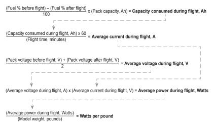
The "LiPo Performance Estimator" spreadsheet, which simplifies these calculations, can be downloaded from <a href="https://www.fmadirect.com/tech\_data/techdocs/">www.fmadirect.com/tech\_data/techdocs/</a>.
