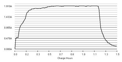
With the 1.0C Auto Current Mode, a fully discharged pack is charged to its nominal capacity in about 60 to 80 minutes, depending on the state of imbalance. Auto Current Mode takes into account a pack's starting charge level, so topping off a 50% discharged pack takes only about 30 minutes.
